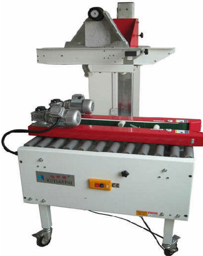
Typical side belt arrangement
