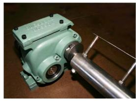
omb Boxes. We are the only source for the original Duesberg comb boxes. These fit all existing cards, are oil-less, and are extremely heavy duty for the highest speed applications. Using these comb boxes you no longer have to worry about oil damage to fibers or fabrics, and save the expense of oil. We have new units, a full assortment of spare parts, and can even repair your old comb boxes.
