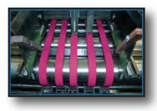
Todays folder/gluer machines run at very high speeds and with the abrasive nature of paperboard, a lot of stress can be put on the belts and the splices. Poor performing belts hurt your quality and efficiency.
